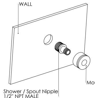
1A. Detach the mounting plate from the backside of the shower head/ spout by unscrewing the two allen screws (mounting screws) located on the bottom side of shower head/spout B (refer to parts list view)
