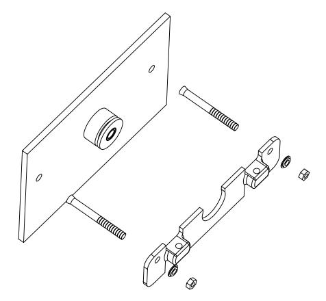
3A. Drill wall with a hole size of 21/64" with a maximum depth of 1 11/32". This depth will allow the lock nut to fasten the mounting plate until it braces the wall.
