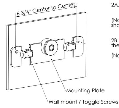
2A. Align the mounting plate to the wall using the mounting guide and position it as desired.
